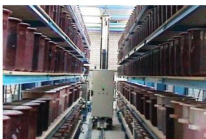
Multiple axis robot for handling buckets with fluids in a two sided storage system.
